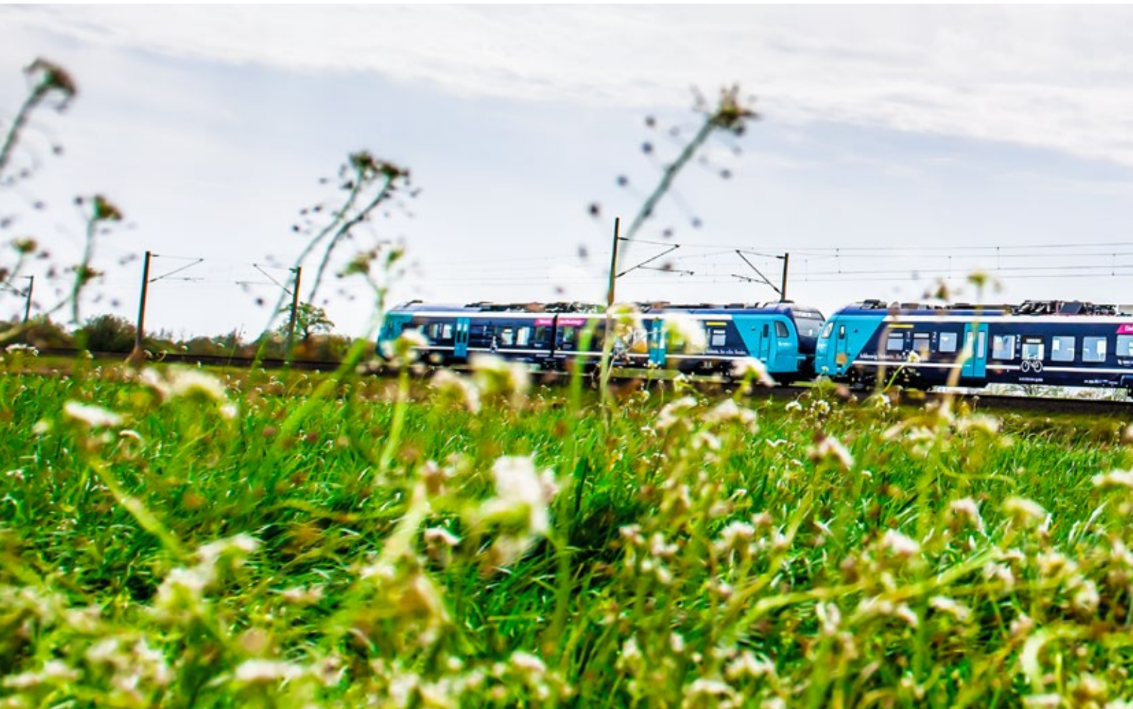
The FLIRT Akku is the battery-operated version of Stadler’s FLIRT model.
