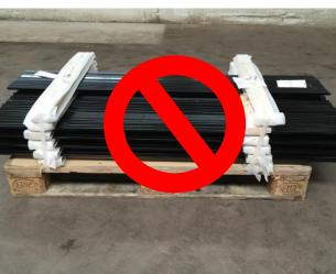
The supply parts must not exceed the outside contour of the load carrier!
