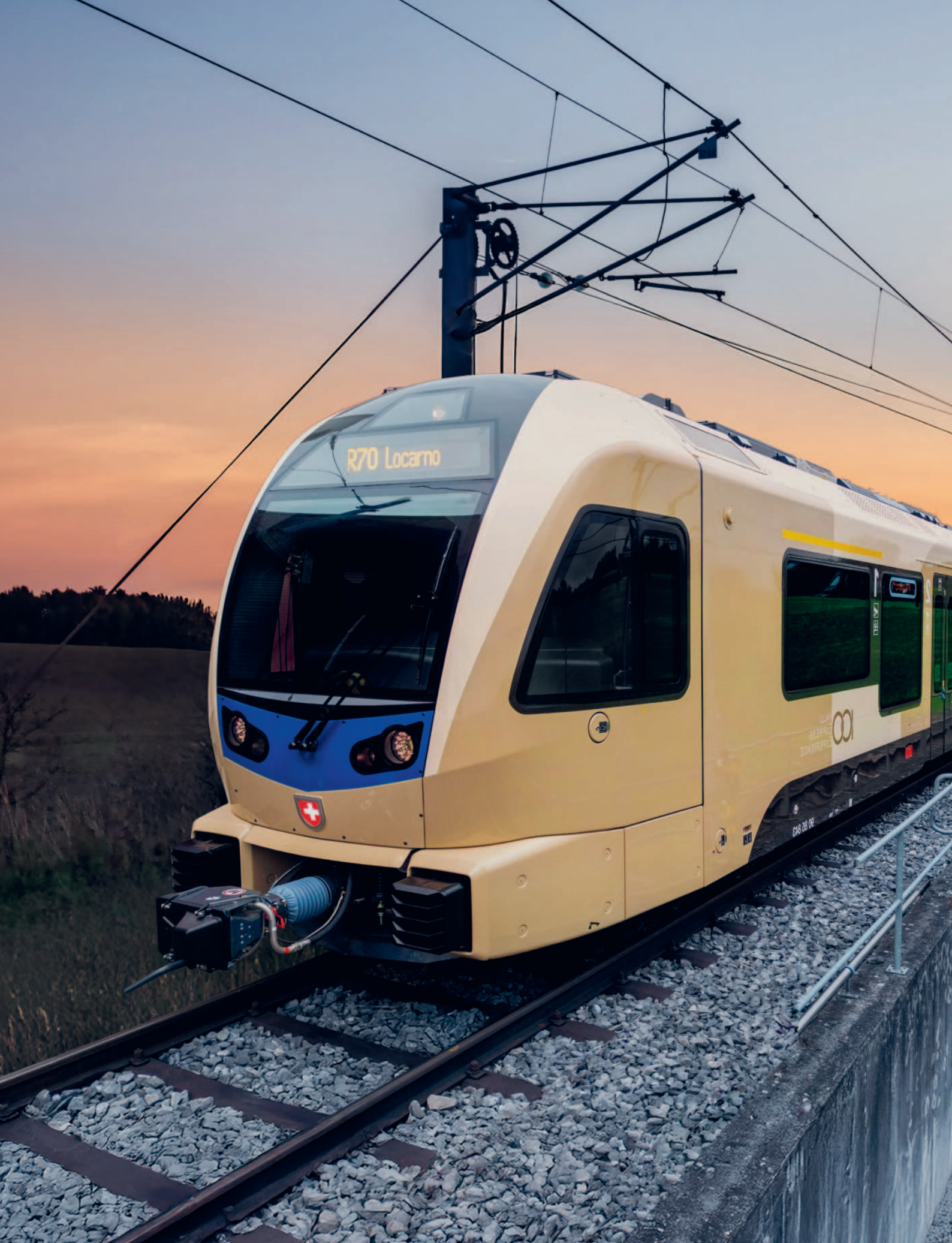
Stadler is building the new electric metre-gauge multiple unit for the famous Centovalli Railway.
