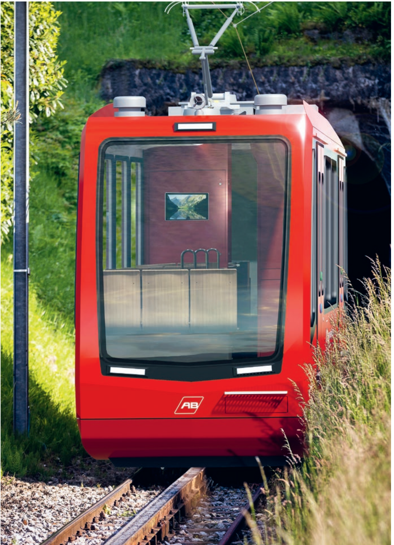
The new vehicle for Appenzeller Bahnen will be the world's first fully automated overland adhesion/rack-and-pinion rail vehicle
