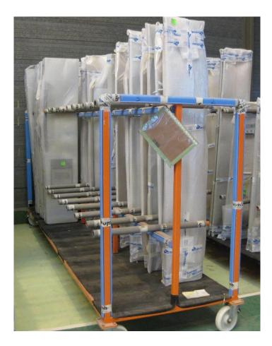
When the door braces are arranged on the transport structure, they should be properly secured in order to avoid movement that could cause blows, scratches, etc.
