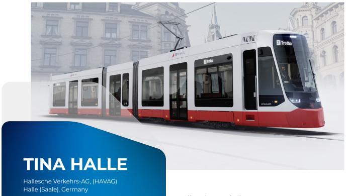
Hallesche Verkehrs-AG, transport operator in Halle, has commissioned Stadler with the delivery of a total of 56 TINA low-floor light rail vehicles of the latest generation.
